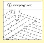
Install the new floor at ninety degrees to the existing subfloor. The crawl space under the plank floor must be sufficiently ventilated. Remove any obstacles and make sure there is sufficient ventilation (minimum 4 cm² (1/2") total ventilation openings per m² (40") of floor). The moisture content of the wood must not exceed 10%.
