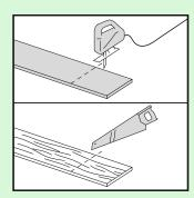
Start with the first plank that will be installed in the corner. Remove the click profile on both the long and the short side of the plank by sawing. For other planks of the first row (not in the corner), remove the click profile on the long side that will be directly next to the wall. Any side of a plank that is directly next to a wall, must have its click profile removed, in order to ensure the required expansion gap.
