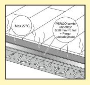
The moisture content of the subfloor must be less than 2,5%CM / 75%RH (cement screed) or less than 0,5%CM / 50%RH (anhydrite screed - subfloor). In the case of floor heating, results must be respectively 1,5%CM / 60%RH and 0,3%CM / 40%RH.
