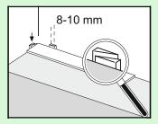
Of course we also need to saw the panels. To obtain a clean cut, the pattern side should face down when you use a jigsaw, sabre saw or circular handsaw and up when you use a handsaw or a crosscut saw. Ensure that the end joints of the panels in two successive rows are never in line.
