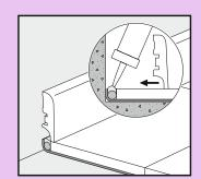
Tip: To make work more cleaner it can be easy to put a tape on the floor before applying the PG Aqua Sealant. This tape can be removed immediatly after applying the PG Aqua Sealant. Spilled PG Aqua Sealant can be removed easily when it is dry.
