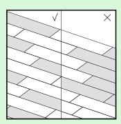
First install the underlay, per width and gradually as you progress. It is vital that you use underlays to smooth any unevenness in the base floor. The smooth top surface makes installing the laminate panels easier and ensures ample expansion afterwards. You can find more information about Pergo underlays and how to install them on the underlay packaging or at your dealer.
