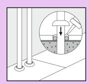
To secure extra water protection around the perimeter of the floor and avoid water to enter underneath the panels, apply the flexible PG Aqua Sealant up to the wall base, thresholds, door frames, pipe covers etc.
