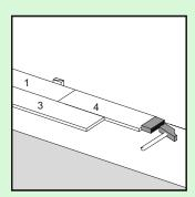
In places where it is too difficult to install the planks with the tapping block (e.g. against the wall), you can tap them together using the pulling iron and a hammer.
