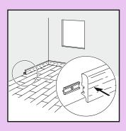
When sawing the panels make sure that the expansion joint under the door is at least 10 mm. If you cannot lift the panel, use the tapping block or pulling iron and hammer to tap the panels together when the planks are flat on the floor.
