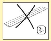
Check whether the old skirting can be removed. You can leave the wall skirting boards in place and finish the floor with Pergo profiles.
