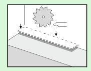
Put the plank with sawn off sides against the walls. Put spacers from the installation kit between the planks and the wall. This will ensure that your expansion joint is wide enough: 8 to 10 mm (5/16" to 3/8").
