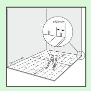
Make sure the panels are mixed sufficiently when you install them, so that you do not end up with too many identical, light or dark panels next to eachother. To obtain the best visual effect, it is best to fit the floorboards in the direction of the longest wall and parallel to the incidence of light.
