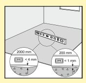
After checking the subfloor for unevenness, carefully vacuum the entire surface. Make sure that the floor base is flat, clean, firm, and dry. To avoid risk of squeaking, secure any loose particleboard, OSB, fiberboard, timber planks etc. with screws.
