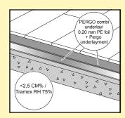
Make sure the subfloor is level. Any unevenness greater than 4 mm over the length of 2 meter must be smoothed out. The same applies to any unevenness of more than 1 mm over a length of 20 cm. This rule does not cope to national reguations about levelling.
