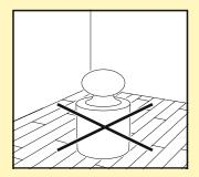
Pergo laminate flooring is designed to be installed as a floating floor to allow natural expansion and contraction with changes in temperature and humidity. To achieve the benefits of a floating floor and to avoid possible gaps, squeaking etc. never fasten the floor with nail, screws, silicone etc.
